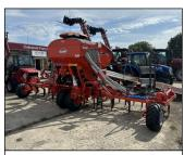
w Kuhn Megant 602 R, 6m mounted drill, direct straight tine coulters, 1800l tank, hyd drive fan, ISOBUS control. £POA
