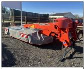
New Kuhn FC 314 D-FF rear mower conditioner, 3.1m ww, FAST-FIT blades, horizontal fold, steel tine conditioner. £POA
