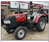
w Case IH Farmall 55A, 2wd, 8 x 8 Powershuttle, 2 mechanical spool valves, 540 PTO, ROPS.
