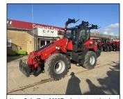
New Schaffer 8620T pivot steer loader, 40kph hydrostatic, air con, 4200kg, 5.2m, boom sus, pin and cone carriage.
